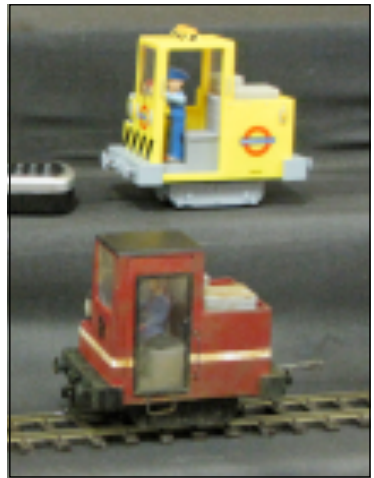
Left Above: Paul Mackinnon's conversion of a cheap radio-controlled toy car into a gandy dancer with an LED headlight taken from a cheap torch. (Headlight and tail light use the no-longer-needed left and right turn buttons on the transmitter.) Button-pressing finger courtesy of Bob the Builder.
